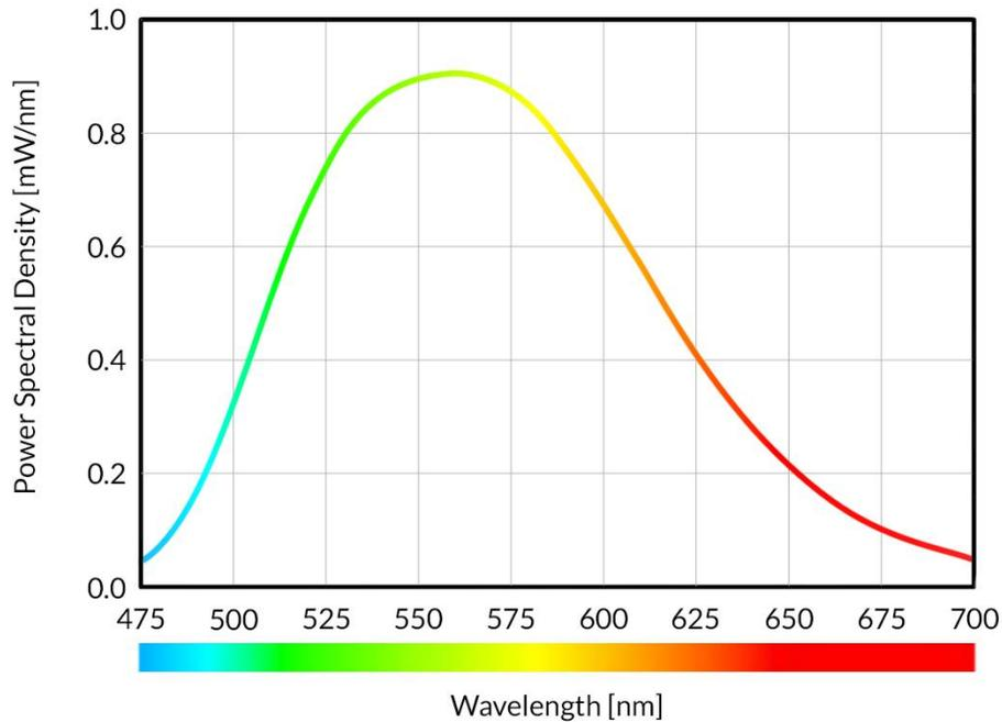
Output power spectral density (PSD) of a *Ce:YAG Fiber Light Source* using a 200  $\mu\text{m}$ , 0.53 NA optical fiber. Power and irradiance specifications are respectively given in Table 13 and 14.
