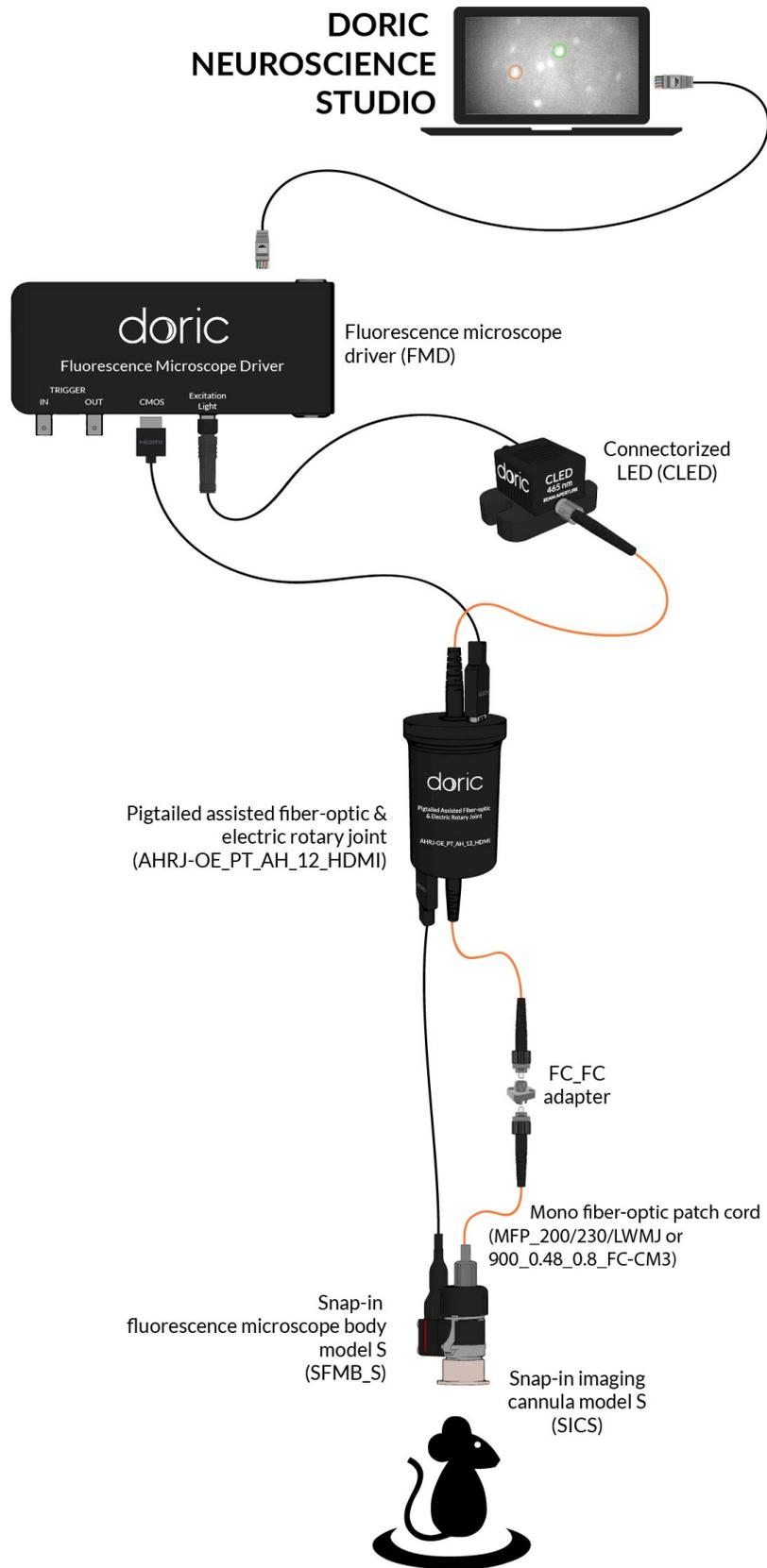
Basic Fluorescence Microscopy System for Surface Imaging of GCaMP6
