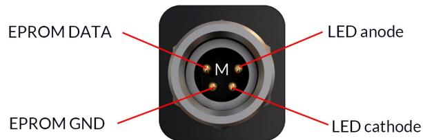
Connectorized LED male pinout
