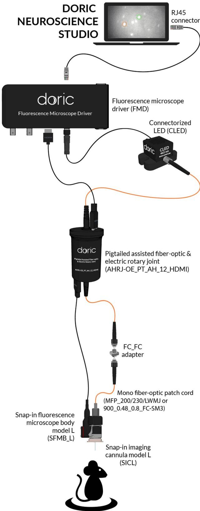
Basic Fluorescence Microscopy System for Deep-brain Imaging of GCaMP6
